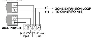
**CAUTION:** APPLY POWER AFTER ALL CONNECTIONS HAVE BEEN MADE/ INSPECTED. DO NOT COIL EXCESS WIRING INSIDE DETECTOR.
